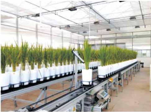
Plant cultivation on moving field conveyer system and various imaging platforms in Nanaji Deshmukh Plant Phenomics Centre at ICAR-IARI, New Delhi
