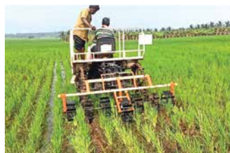
Multi-row rotary weeder attachment to rice transplanter
