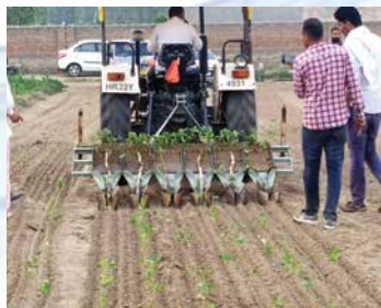
Tractor operated Paper-tape Vegetable Transplanter
