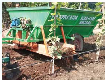
Trencher-cum-FYM applicator for grape orchards
