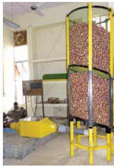
Modular onion storage structure
